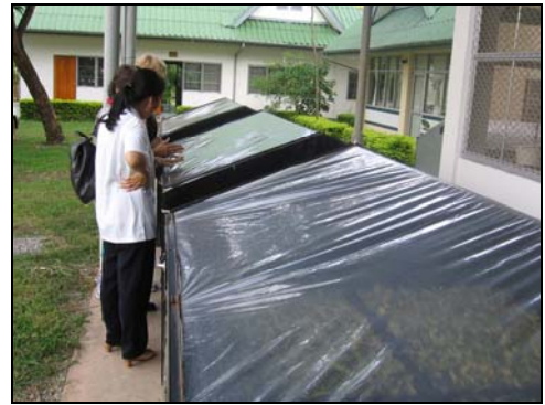
Figure 1. Solar Driers used to preserve farm products and prepared foods
